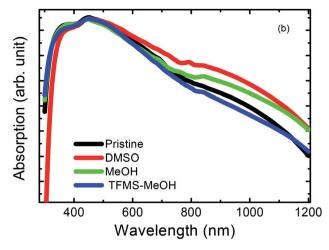
Fig. 3 (a) The S 2p XPS spectra of glass substrate, pristine and TFMS-MeOH treated PEDOT:PSS thin film. (b) The absorption spectra of PEDOT: PSS thin films with and without treatment.
