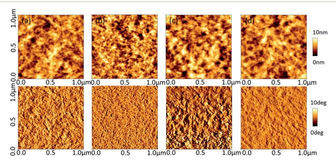
Fig. 4 The AFM surface morphology of PEDOT:PSS thin films with different solvent treatment: (a) pristine, (b) DMSO treatment, (c) MeOH treatment, (d) TFMSA-MeOH treatment. The upper and lower row images are height images and phase images, respectively.
