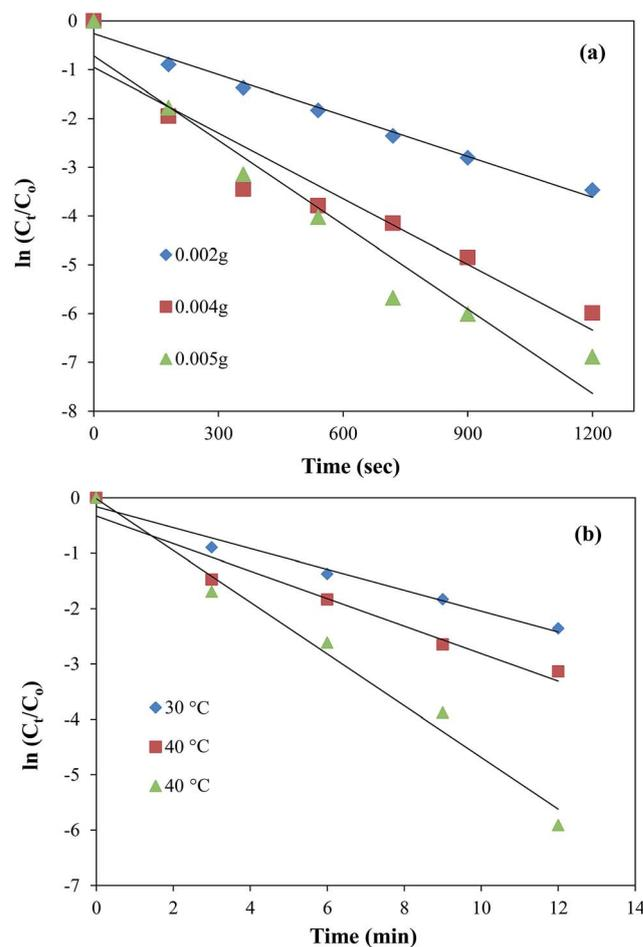
Fig. 8 Dependence of  $k_{app}$  on (a) the amount of catalyst at 30 °C and (b) temperature. Reaction conditions; 0.5 mM aqueous solution of 2-nitroaniline = 50 ml,  $\text{NaBH}_4 = 0.1$  g, graphene oxide-gold catalyst = 5 mg, 100 rpm.
