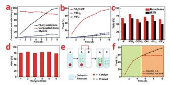
Fig. 3 (a) Time-dependent catalysis by the Pd<sub>1</sub>/H-ZIF. (b) Reaction performances for Pd<sub>1</sub>/H-ZIF, Pd/C and PdCl<sub>2</sub> in dimerization of phenylacetylene to generate a conjugated diene. (c) Catalytic performances for dimerization of substituted phenylacetylene over the Pd<sub>1</sub>/H-ZIF. (d) The recyclability of Pd<sub>1</sub>/H-ZIF. (e and f) Hot filtration test.
