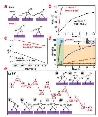
Fig. 4 (a and b) Different routes in the reaction process. (c) Arrhenius plot of the different reaction routes for Pd<sub>1</sub>/H-ZIF. (d) The influence of different atmospheres in different routes. (e) Energies of intermediates and transition states in the mechanism of phenylacetylene dimerization at the Pd<sub>1</sub>/H-ZIF from DFT calculations.
