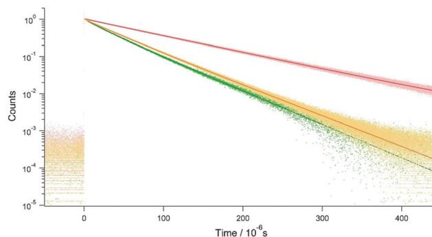
**Fig. 6** Phosphorescence decays of PtCP-fixed glass (red) and PtCP solutions in THF deoxygenated by Ar bubbling (green) and by freeze-pump-thaw cycles (orange), together with fitting curves (solid lines, see text). The concentration of PtCP was 75  $\mu\text{M}$  for all samples. The excitation energy was 7.3  $\mu\text{J}$  per pulse.
