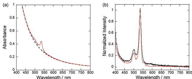
**Fig. 2** UV-vis absorption spectra of (a) PtCP-fixed porous glass with a concentration of 77  $\mu\text{M}$  (red line) and blank porous glass (dashed black line). (b) Normalized UV-vis absorption spectra of PtCP obtained by subtracting the blank porous glass from the PtCP-fixed porous glass (solid black line) and PtCP in THF with a concentration of 7.9  $\mu\text{M}$  (solid red line).
