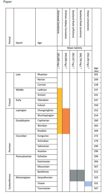
Fig. 2 Stratigraphic chart annotated with mean salinities (mg L<sup>-1</sup>) of FP and produced water data by source formation for the UK.
