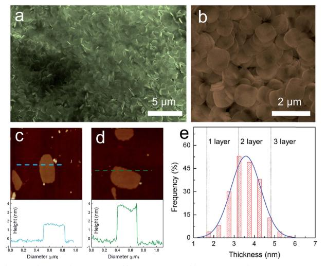
Fig. 8 Synthesis of 2D ultrathin CsPbBr<sub>3</sub> nanosheets: (a) low-magnification and (b) high-magnification SEM images. AFM image and height profile of (c) monolayer and (d) bilayer CsPbBr $_3$  nanosheets with a thickness of 1.6 and 3.3  $\pm$  0.2 nm, respectively. (e) Thickness distribution histograms for CsPbBr<sub>3</sub> nanosheets prepared through solution-phase synthesis. Reprinted from ref. 79, copyright 2016, Advanced Materials.
