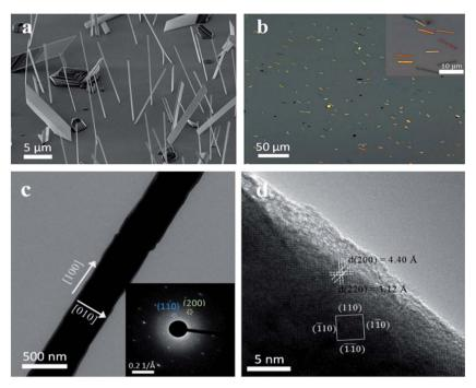
Fig. 5 (a) SEM image of  $Pbl_2$  nanowires grown on the silicon substrate. (b) Optical microscopy image of  $CH_3NH_3Pbl_3$  nanowires on the silicon substrate. Inset in (b) is the magnified image. (c) TEM and (d) HRTEM images of  $CH_3NH_3Pbl_3$  nanowire. Inset in (c) is its corresponding SAED pattern. Reprinted with permission from ref. 39, copyright 2015, American Chemical Society.
