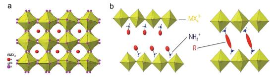
Fig. 1 Structure of 3D and 2D perovskites: 33 (a) structure of AMX3 3D perovskite; (b) structure of layered perovskites with (left) monoammonium (RNH<sub>3</sub><sup>+</sup>) or (right) diammonium (<sup>+</sup>H<sub>3</sub>N-R-NH<sub>3</sub><sup>+</sup>) organic cations.
