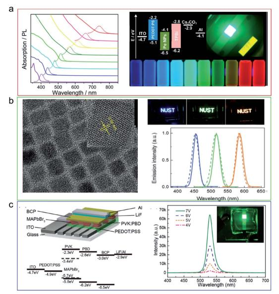
Fig. 12 Low dimensional perovskite in LED applications. (a) LED from  $CH_3NH_3PbX_3$  quantum dots. (b) LED from  $CsPbX_3$  quantum dots. (c) LED from  $CH_3NH_3PbX_3$  nanoplatelets. Reprinted with permission from ref. 17, 90 and 91.
