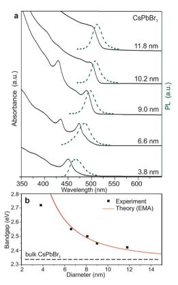
Fig. 10 (a) Quantum-size effects in the absorption and emission spectra of 5–12 nm CsPbBr<sub>3</sub> NCs. (b) Experimental *versus* theoretical (effective mass approximation, EMA) size dependence of the band gap energy. Reprinted with permission from ref. 49.
