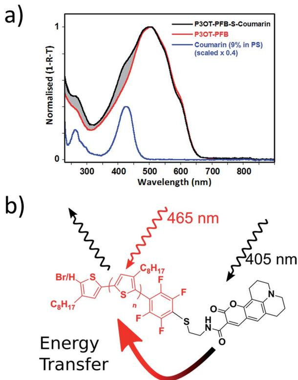
Fig. 4 (a) Peak normalized thin-film UV-visible spectra (obtained from recording both specular reflection and transmission) for P3OT-PFB, P3OT-PFB-S-Coumarin<sub>343</sub>, and Coumarin<sub>343</sub>-SH dispersed in a polystyrene matrix (9 wt%). Films spun from THF (5 mg mL<sup>-1</sup>) (b) schematic representation of P3OT-PFB-S-Coumarin<sub>343</sub> illustrating the likely route of interchain energy transfer and emission from P3OT.
