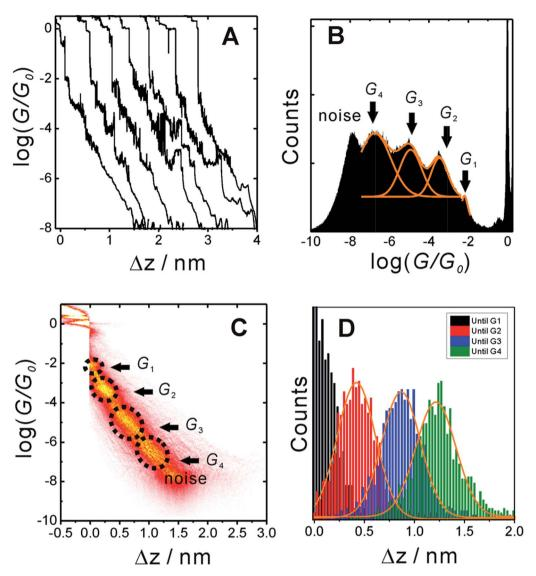
Fig. 3 (A) Typical individual conductance *versus* relative displacement distance traces of **TP1** recorded in MCBJ experiments in 1,3,5-trimethyl benzene (TMB)/tetrahydrofuran (THF) (4 : 1, v/v) containing 0.1 mM of the target molecules. (B) 1D logarithmic conductance histograms constructed from more than 1000 individual curves and recorded with a bias voltage of 0.10 V. (C) 2D conductance histogram. (D) Characteristic length 1D histograms analysed for  $G_1$ ,  $G_2$ ,  $G_3$  and  $G_4$ .
