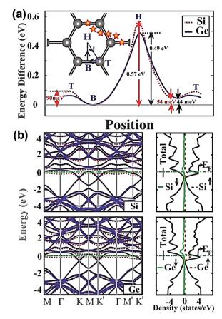
Fig. 1 (a) Binding energy of Si and Ge adatoms in different sites, and their migration path. The adsorption sites were divided and named, top (T), bridge (B) and hollow (H), as shown in the map inserted in (a). (b) Energy band structure and total density of states of Si and Ge atoms adsorbed to graphene in the  $(4 \times 4)$  supercell. Reprinted with permission from ref. 35. Copyright 2010 American Institute of Physics.
