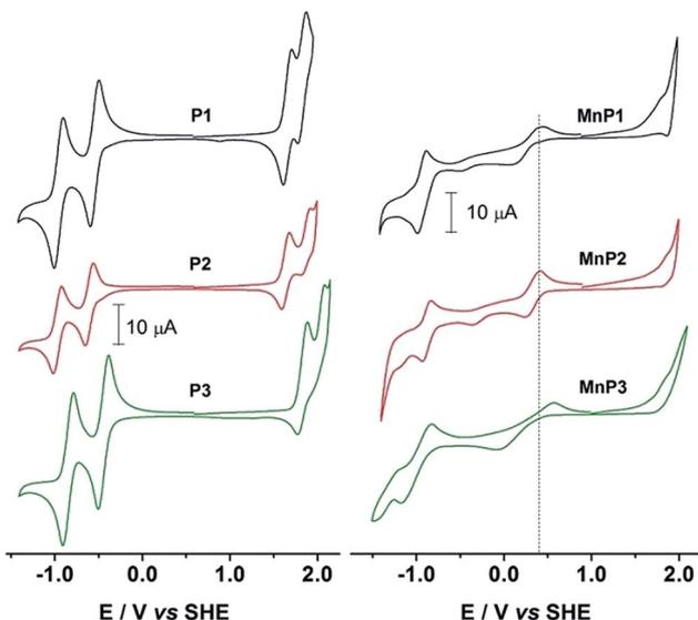
Fig. 2 Cyclic voltammograms of  $\text{H}_2\text{P}$  and  $\text{MnP}$  in dichloromethane containing  $0.1 \text{ mol L}^{-1}$   $\text{TBAPF}_6$ . Scan rate at  $100 \text{ mV s}^{-1}$ . Initial anodic scan.
