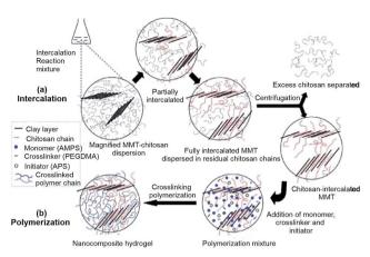
Fig. 9 Preparation of poly(AMPS)/chitosan/MMT nanocomposite hydrogels: (a) intercalation reaction, (b) crosslinking polymerization. Reproduced from ref. 83. Copyright (2009), with permission from Wiley-VCH.
