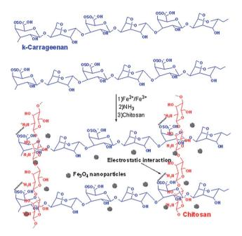
Fig. 8 Scheme for the preparation of magnetic carrageenan/chitosan complex. Reprinted from ref. 79. Copyright (2017), with permission from Flsevier
