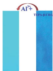
Fig. 8 Fluorescence of filter paper in a solution of L and L + \text{Al}^{3+} under UV light.
