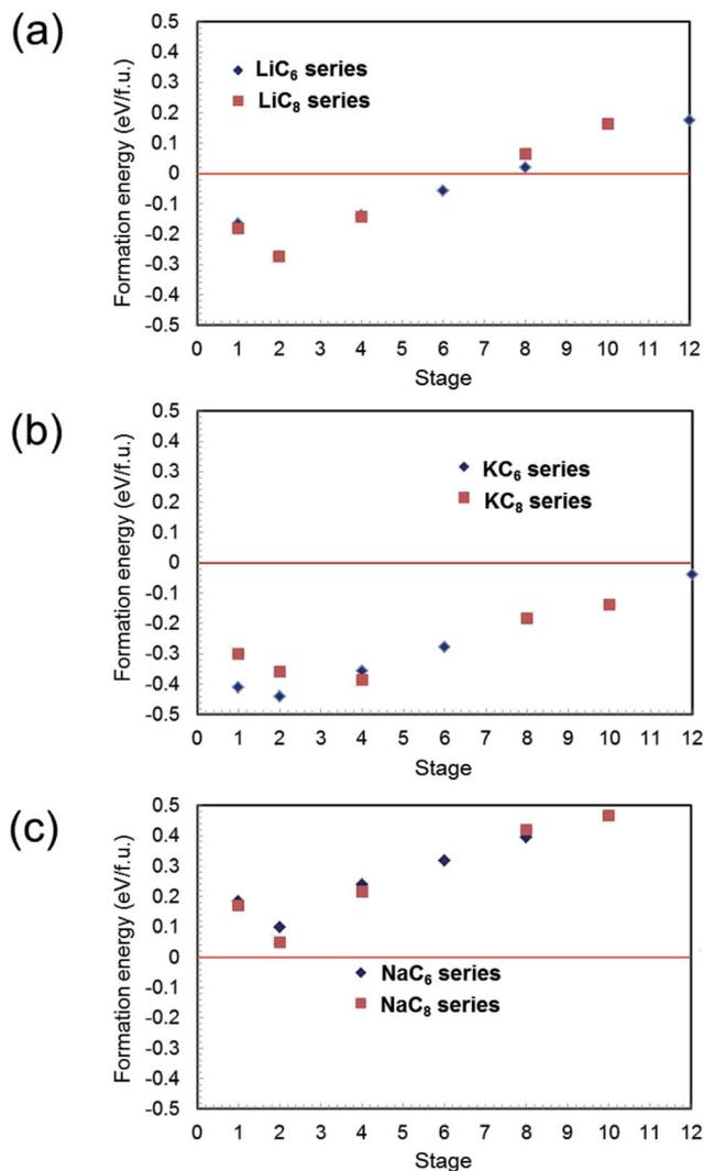
Fig. 1 Calculated formation energies of AM-GICs (AM = Li, Na and K) as a function of stage number for AMC<sub>6</sub> and AMC<sub>8</sub> series: (a) Li-GIC, (b) K-GIC and (c) Na-GIC.
