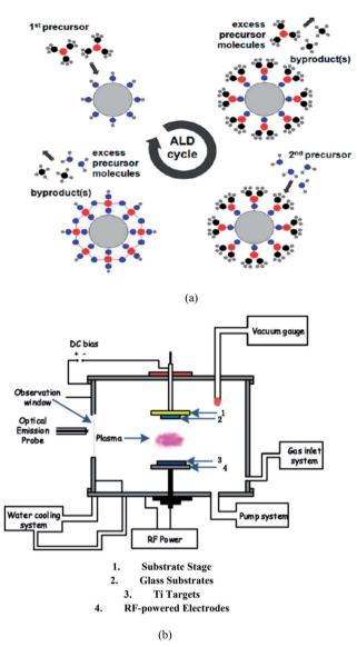
Fig. 11 Schematic representation of various seeding methods: (a) ALD<sup>83</sup> and (b) RF magnetron sputtering.<sup>84</sup>
