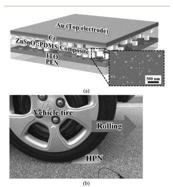
Fig. 18 (a) Schematic diagram of ZnSnO<sub>3</sub>:PDMS-based flexible hybrid PENG. (b) Experimental setup used for the generation of power from the hybrid PENG under a rolling vehicle tire.200
