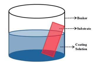
Fig. 14 Schematic of dip coating technique
