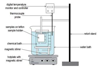
Fig. 8 Experimental setup used for chemical bath deposition.<sup>68</sup>
