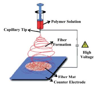
Fig. 12 Schematic illustration of a typical laboratory setup for conventional electrospinning with vertical feeding of the solution.<sup>90</sup>
