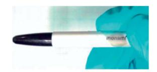
Fig. 22 Fully rollable graphene-based NG. 103
