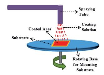
Fig. 15 Experimental setup used for spin coating on a substrate
