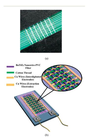
Fig. 19 (a) Photograph of a fabric nanogenerator (FNG). (b) Structure of the FNG.  $^{248}$
