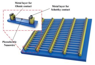
Fig. 4 Basic structure of LING
