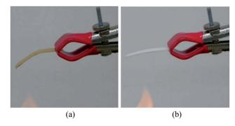
Fig. 17 Thermal stability of (a) paper-based nanogenerator and (b) polymer-based nanogenerator.<sup>243</sup>
