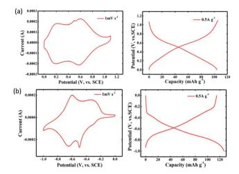
Fig. 15 CV and charge/discharge curves  $(0.5 \text{ A g}^{-1})$  for (a) polytriphenylamine cathode, (b) 1,4,5,8-naphthalenetetracarboxylic dianhydride-derived polyimide anode. Reproduced with permission from ref. 186, copyright 2017, John Wiley and Sons.
