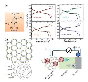
Fig. 18 (a) Structure of Li<sub>2</sub>DAnT and voltage profiles of Li<sub>2</sub>DAnT when hosting different anions. <sup>197</sup> (b) Porous organic anion host of having a honeycomb structure with a pore diameter of 1.4 nm, and (c) discharging process with  ${\rm ClO_4}^-$  anions move out from the organic host. Reproduced with permission from ref. 198, copyright 2013, Nature Publishing Group.
