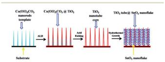
Fig. 9 Schematics of the fabrication process of TiO<sub>2</sub> nanotube@SnO<sub>2</sub> nanoflake core-branch nanostructures. Reproduced with permission from ref. 134, copyright 2014, Elsevier.
