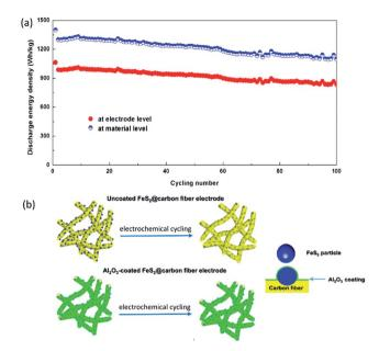
Fig. 13 (a) Cycling stability at material level (W h kg<sub>FeS</sub>, <sup>-1</sup>) and electrode level (W h kg<sub>FeS<sub>2</sub></sub> electorde<sup>-1</sup>) for Al<sub>2</sub>O<sub>3</sub>-coated FeS<sub>2</sub>@carbon fiber electrode; (b) illustration of mechanisms for the enhanced cycling stability by Al<sub>2</sub>O<sub>3</sub> coating. Reproduced with permission from ref. 180, copyright 2016, American Chemical Society.
