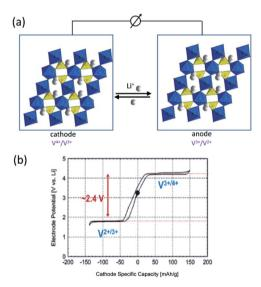
Fig. 19 (a) Schematic illustration of a symmetric LIB with two redox couples of  $V^{4+}/V^{3+}$  and  $V^{3+}/V^{2+}$  in the LiVPO<sub>4</sub>F. Reproduced with permission from ref. 201, copyright 2011, American Chemical Society. (b) (De)lithiation reactions for a Li/LiVPO<sub>4</sub>F cell from 1.6 to 4.4 V showing two potential steps with a gap of about 2.4 V. Reproduced with permission from ref. 202, copyright 2013, American Chemical Society.
