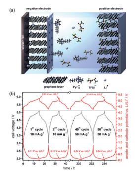
Fig. 17 (a) Schematic illustration of a dual-ion battery using graphite as both cathode and anode, with the formation of a stable SEI layer at the negative graphite electrode. (b) Cathode potential, anode potential (red curves) and cell voltage (dotted black curve) profiles. Reprinted with permission.<sup>193</sup>
