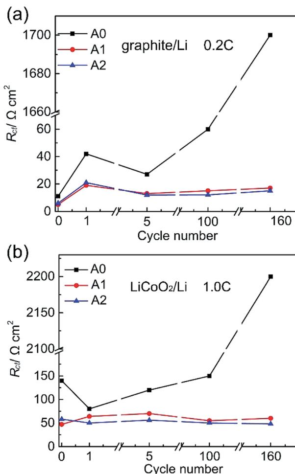
Fig. 2 EIS spectra of the graphite/Li and  $\text{LiCoO}_2/\text{Li}$  half-cells with electrolytes A0, A1 and A2, after storage for 24 h, 1st, 5th, 100th and 160th cycles at 25 °C. Frequency range of  $10^{-2}$  Hz to  $10^5$  Hz with a potential amplitude of 5 mV. (a) The change of the charge-transfer resistances ( $R_{ct}$ ) in the graphite/Li cells. (b) The change of  $R_{ct}$  in the  $\text{LiCoO}_2/\text{Li}$  cells.
