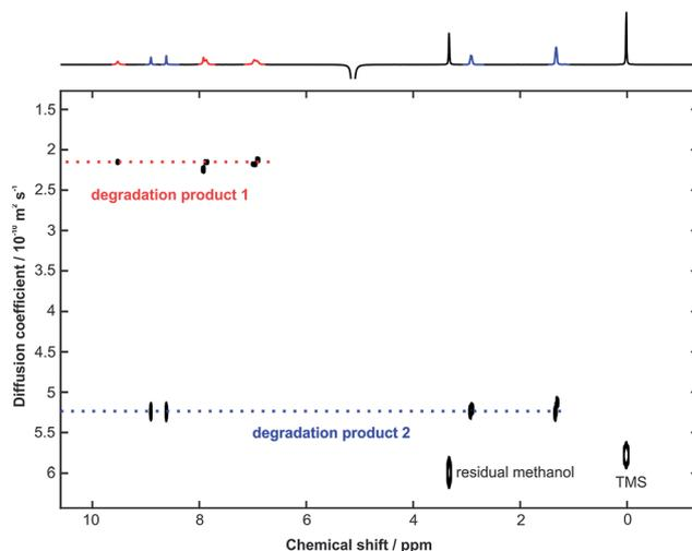
Fig. 4 500 MHz  $^1\text{H}$  DOSY spectrum, with the least attenuated 1D spectrum shown at the top, acquired after 17 h of monitoring of a sample containing 24 mM voriconazole, and 48 mM NaOH in  $\text{CD}_3\text{OH}$  at 10  $^\circ\text{C}$ .
