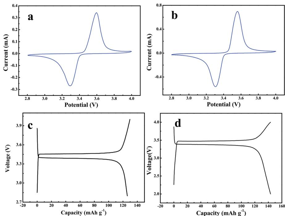
Fig. 9 (a) CV curve of  $\text{LiFePO}_4$  testing with GPE. (b) CV curve of  $\text{LiFePO}_4$  cathode with liquid electrolyte. (c) Charge–discharge curves of  $\text{LiFePO}_4$  testing with GPE at  $80 \text{ mA g}^{-1}$ . (d) Charge–discharge curves of  $\text{LiFePO}_4$  testing with liquid electrolyte at  $80 \text{ mA g}^{-1}$ .
