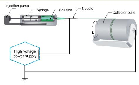
Fig. 2 Schematic of a typical setup for electrospinning
