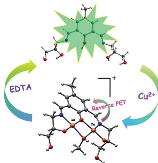
Scheme 2 Schematic illustration of proposed mechanism for the fluorescence changes of chemosensor (H<sub>5</sub>dpm) upon addition of Cu<sup>2+</sup>.
