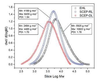
Fig. 2 The GPC curves of EHL, SCEP-RL and SCEP-DL samples.
