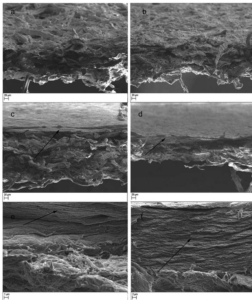
Fig. 3 SEM images of sludge (a) sludge–CNF<sub>SL</sub> (b) support layers. Bilayered membranes having S/CNC<sub>BE</sub> (c and e) and S–CNF<sub>SL</sub>/CNC<sub>BE</sub> (d and f) compositions with different resolutions were also shown. Layered structure of membranes is clearly visible having upper dense functional layer (as indicated by arrow) and lower loose network made up of sludge fibers or S–CNF<sub>SL</sub> mixture.
