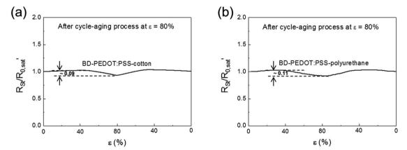
Fig. 8 The  $R_{\rm St}/R_{\rm 0,sat'}$  values of (a) BD-PEDOT:PSS-cotton and (b) BD-PEDOT:PSS-polyurethane during a cycle of 80% loading after performing the cycle-aging process at  $\varepsilon = 80\%$
