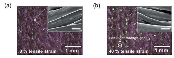
Fig. 6 Optical and SEM images of the BD-PEDOT: PSS-cotton before (a) and after (b) loading 40% tensile strain. The scale bar of the SEM image is  $10 \mu m$ .
