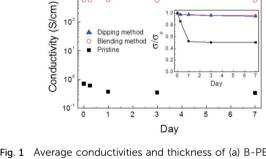
Fig. 1 Average conductivities and thickness of (a) B-PEDOT:PSS and (b) D-PEDOT:PSS. (c) Electrical stability tests of pristine-, B-, and D-PEDOT:PSS under constant conditions (relative humidity and temperature: 40% and 22.5 °C, respectively) for 7 days. The inset shows the normalised conductivity with respect to time.
