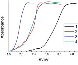
Fig. 5 UV-Visible spectra of compounds 1–4. The following  $E_{\text{onset}}$ values were determined by means of the tangent method: 2.9 eV (1); 2.4 eV (2); 1.7 eV (3); 2.1 eV (4). Note that the onset of absorption for compound 2 is intrinsically red-shifted due to the beginning of decomposition of the very sensitive compound during sample preparation; for this, only the sharply ascending part of the curve was used to determine the optical gap.
