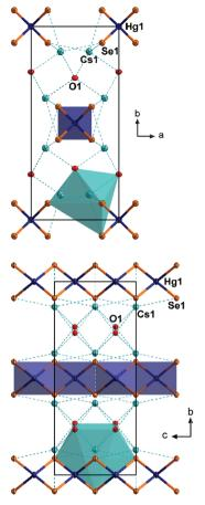
Fig. 2 Fragments of the crystal structure of 2, viewed along  $\langle 001 \rangle$  (top) and  $\langle 100 \rangle$  (bottom). The coordination polyhedra around the Hg atoms of the central strand and around one Cs atom are shown. All atoms are drawn with displacement ellipsoids at the 50% probability level.
