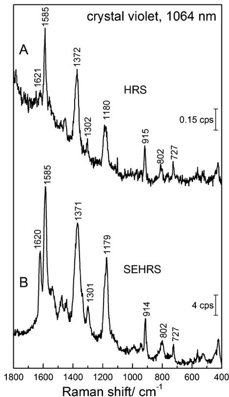
**Fig. 10** (A) Hyper Raman spectrum of crystal violet dye and (B) surface enhanced hyper Raman spectrum of crystal violet in the local field of silver nanostructures. Excitation: 1064 nm (A and B), photon flux density:  $6.8 \times 10^{27}$  photons  $\text{cm}^{-2} \text{s}^{-1}$  (A) and  $1.4 \times 10^{27}$  photons  $\text{cm}^{-2} \text{s}^{-1}$  (B), acquisition time: 8 min (A) and 1 min (B), crystal violet concentration:  $1 \times 10^{-3}$  M (A) and  $1 \times 10^{-5}$  M (B).
