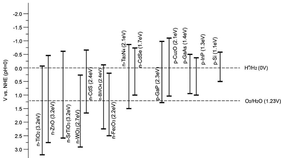
Fig. 9 Band positions of various semiconductors with respect to the redox potentials of water splitting at pH = 0.
