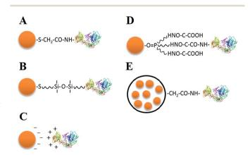
Fig. 2 Common bioconjugation strategies of QDs, including connection between carboxyl and amino (-COOH and -NH2) functional groups of bifunctional molecules (A), functional group linkage of typical silane compounds (B), electrostatic interaction (C), linkage between hydrophilic and hydrophobic groups (D), and the use of functionalized microbeads as conjugation media (E). A, B, and D belong to the category of covalent linkage strategies.
