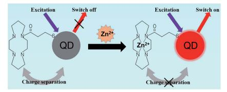
Fig. 6 Schematic principle of zinc ion nanosensors. Conjugation of QDs and azamacrocycles causes charge separation and guenching of QDs. The complexation of Zn(II) with the ligand changes the energy level on the ligand, which prevents the charge separation and leads to the fluorescence recovery of QDs. Reproduced from ref. 106 with permission. Copyright © 2008, American Chemical Society.
