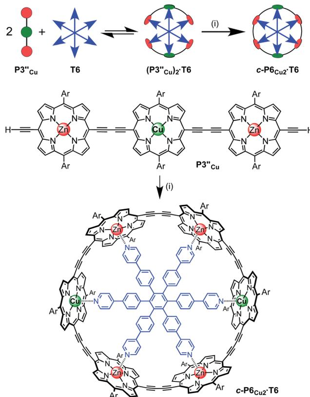
**Scheme 2** Synthesis of  $c-P6_{Cu_2} \cdot T6$ . Two representations of the synthetic route used to prepare  $c-P6_{Cu_2} \cdot T6$ . Reaction conditions: (i)  $PdCl_2(PPh_3)_2$ , CuI, 1,4-benzoquinone, *i*-Pr<sub>2</sub>NH,  $CHCl_3$ , 2%. Ar = 3,5-bis(*tert*-butyl)phenyl.
