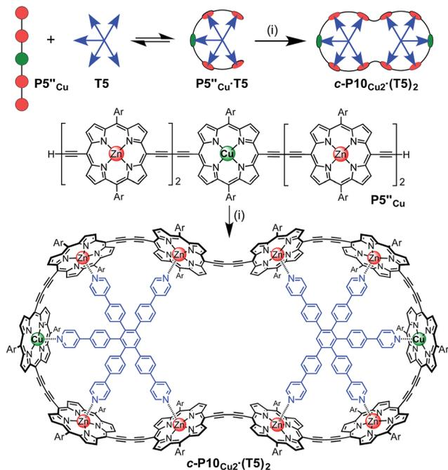
**Scheme 3** Synthesis of  $c\text{-P10Cu}_2(\text{T5})_2$ . Two representations of the synthetic route used to prepare  $c\text{-P10Cu}_2(\text{T5})_2$ . Reaction conditions: (i)  $\text{PdCl}_2(\text{PPh}_3)_2$ ,  $\text{CuI}$ , 1,4-benzoquinone,  $i\text{-Pr}_2\text{NH}$ ,  $\text{CHCl}_3$ , 17%. Ar = 3,5-bis(*tert*-butyl)phenyl.
