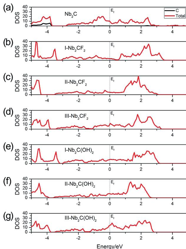
Fig. 2 Total DOS of (a)  $\text{Nb}_2\text{C}$ , (b) I- $\text{Nb}_2\text{CF}_2$ , (c) II- $\text{Nb}_2\text{CF}_2$ , (d) III- $\text{Nb}_2\text{CF}_2$ , (e) I- $\text{Nb}_2\text{C}(\text{OH})_2$ , (f) II- $\text{Nb}_2\text{C}(\text{OH})_2$  and (g) III- $\text{Nb}_2\text{C}(\text{OH})_2$ . The Fermi levels are set to zero.
