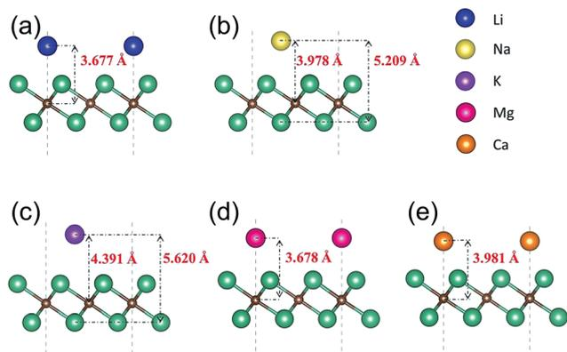
Fig. 4 Side views of the optimized structures of Nb<sub>2</sub>C monolayers after adsorption with (a) Li, (b) Na, (c) K, (d) Mg and (e) Ca.
