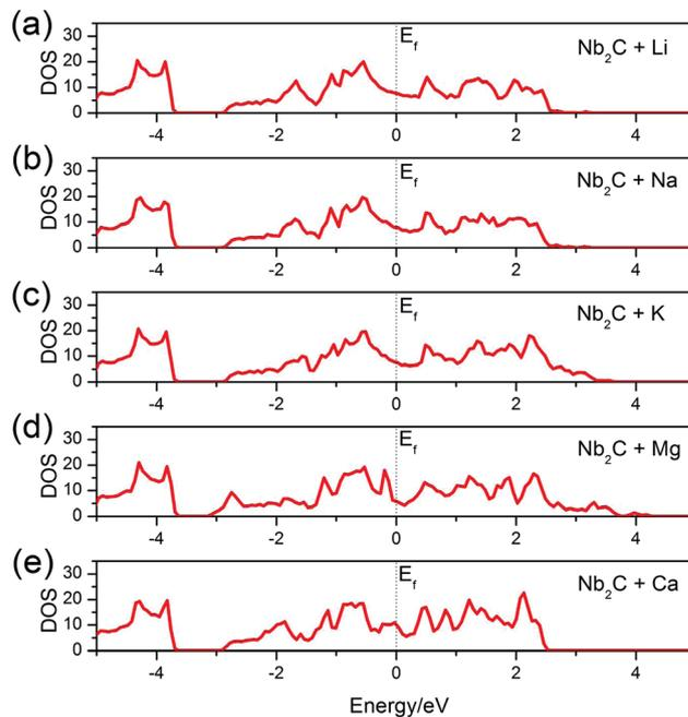
Fig. 5 Total DOS of the bare Nb<sub>2</sub>C monolayer after (a) Li, (b) Na, (c) K, (d) Mg and (e) Ca adsorption. The dotted vertical lines denote the Fermi levels.
