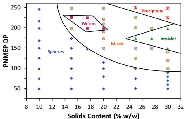
Fig. 5 Phase diagram for a series of PSMA<sub>14</sub>-PNMEP<sub>x</sub> diblock copolymers synthesised by RAFT dispersion polymerisation of NMEP in *n*-dodecane at various concentrations ranging between 10 and 30% w/w solids. Post-polymerisation analysis of each diblock copolymer dispersion by TEM determined the phase boundaries.
