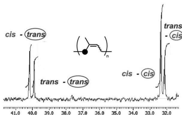
Fig. 1 A part of the <sup>13</sup>C NMR spectrum of polyisoprene synthesized by using the Nd–Mg/Al catalyst system (125 MHz, in CDCl<sub>3</sub>, Table 1, run 4).
