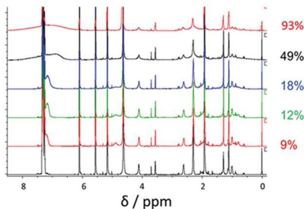
**Fig. 2**  $^1\text{H}$  NMR spectra recorded during the RAFT dispersion polymerization of BzMA at  $70^\circ\text{C}$  in  $d_6$ -ethanol targeting a final diblock composition of PDMA<sub>43</sub>-PBzMA<sub>500</sub>. Monomer conversions were calculated by comparing the integrals of the vinyl monomer to the  $t = 0$  spectrum using TMS as the internal standard.
