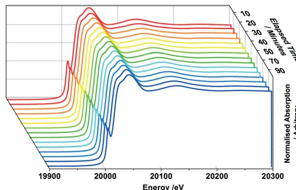
Fig. 7 XANES data over a 90 minute period for 6 ML MoO<sub>x</sub>/Fe<sub>2</sub>O<sub>3</sub> when reacted isothermally at 250 °C under a continuous flow of MeOH/O<sub>2</sub>. XAFS data was collected continuously using 1 minute scans, whilst Mass Spectrometer data was recorded simultaneously, to ensure a reaction was occurring.
