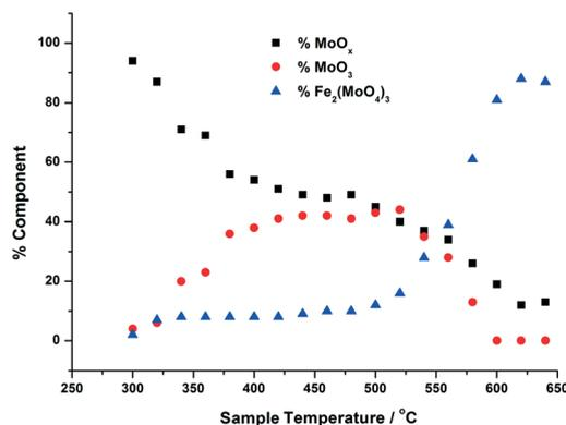
**Fig. 5** Phase composition of  $\text{MoO}_x$ ,  $\text{MoO}_3$ ,  $\text{Fe}_2(\text{MoO}_4)_3$  with increasing calcination temperature, for 6 ML  $\text{MoO}_x/\text{Fe}_2\text{O}_3$ . The calcination was performed as in Fig. 3, and the phase compositions were determined using linear combination analysis of  $\text{MoO}_3$  and  $\text{Fe}_2(\text{MoO}_4)_3$  (Sigma Aldrich) and the dried 6 ML  $\text{MoO}_x/\text{Fe}_2\text{O}_3$ .
