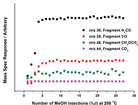
Fig. 8 Online Mass Spectrometry data for 6 ML MoO<sub>x</sub>/Fe<sub>2</sub>O<sub>3</sub>, when reacted isothermally in continuous flow under MeOH/O<sub>2</sub> at 250 °C (see Fig. 7 for details). Selectivity to formaldehyde was 90%. The data has not been normalised to the fragmentation pattern of products produced.
