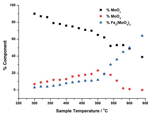
**Fig. 4** Phase composition of  $\text{MoO}_x$ ,  $\text{MoO}_3$ ,  $\text{Fe}_2(\text{MoO}_4)_3$  with increasing calcination temperature, for 3 ML  $\text{MoO}_x/\text{Fe}_2\text{O}_3$ . The calcination was performed as in Fig. 3, and the phase compositions were determined using linear combination analysis of  $\text{MoO}_3$  and  $\text{Fe}_2(\text{MoO}_4)_3$  (Sigma Aldrich) and the dried 3 ML  $\text{MoO}_x/\text{Fe}_2\text{O}_3$ .
