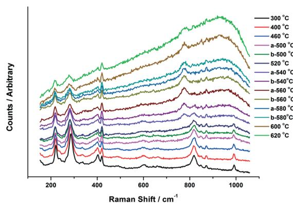
**Fig. 6** Raman data collected *in situ* with combined XAFS/Raman for 6 ML  $\text{MoO}_x/\text{Fe}_2\text{O}_3$ . The catalyst was ramped to 640 °C at a rate of 12 °C  $\text{min}^{-1}$ . Spectra were collected for 20 × 1 second scans using ‘static’ mode, with the grating angle fixed to illuminate the Raman spectrum across the CCD. Temperatures from 300 °C to 620 °C are shown, those labelled (a) are the initial heating ramp, those labelled (b) represent the cooling cycle.
