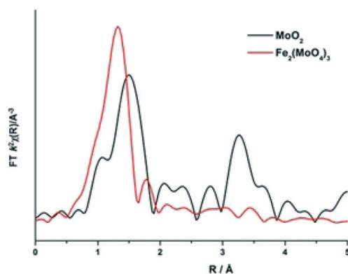
**Fig. 11** Magnitude component of the  $k^2$  weighted Fourier Transform data for MoO<sub>2</sub> and Fe<sub>2</sub>(MoO<sub>4</sub>)<sub>3</sub> (Sigma Aldrich).
