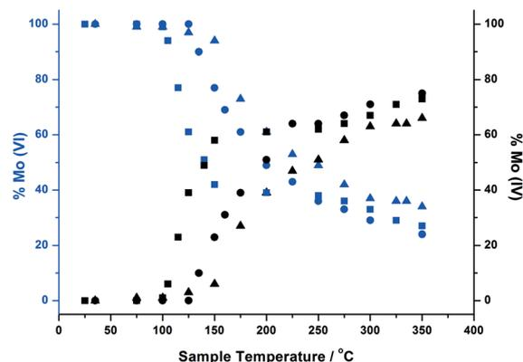
Fig. 9 Oxidation state changes during *in situ* reduction of 1, 3 and 6 ML  $\text{MoO}_x/\text{Fe}_2\text{O}_3$  ascertained through monitoring the change in absorption edge position from  $\text{Mo}(\text{VI})$  to  $\text{Mo}(\text{IV})$ . Reduction studies were carried out in a methanol/He flow whilst heating to 350 °C at a rate of 12 °C  $\text{min}^{-1}$ . XAFS spectra were collected throughout (~1 min per scan). 1 ML = squares, 3 ML = circles, 6 ML = triangles.
