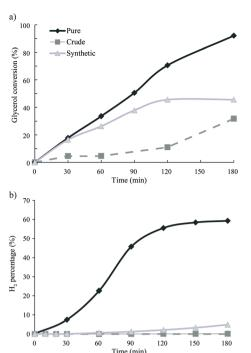
Fig. 1 APR of pure and crude glycerol as a function of time a) glycerol conversion and b) H<sub>2</sub> formation; reaction conditions 1Pt/Al<sub>2</sub>O<sub>3</sub>, 225 °C, 29 bar. 3 h.
