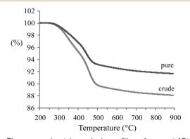
Fig. 4 Thermogravimetric analysis profiles of a spent 1Pt/Al<sub>2</sub>O<sub>3</sub> catalyst after APR of pure and crude glycerol (experiments were performed under flow of air).
