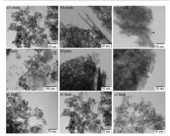
Fig. 2 TEM micrographs of (a) fresh 1Pt/Al<sub>2</sub>O<sub>3</sub> catalyst (a1), spent after pure (a2) and crude glycerol APR (a3); (b) fresh 5Pt/Al<sub>2</sub>O<sub>3</sub> catalyst (b1), spent after pure (b2) and crude glycerol APR (b3), and (c) fresh 5Pt/C catalyst (c1), spent after pure (c2), and crude glycerol APR (c3).
