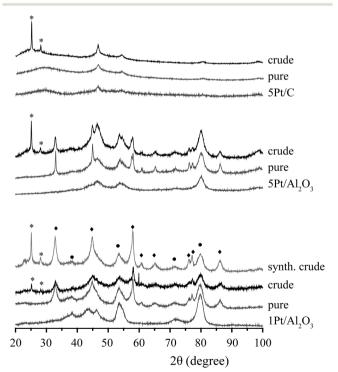
Fig. 6 XRD patterns of  $1Pt/Al_2O_3$ ,  $5Pt/Al_2O_3$  and 5Pt/C catalysts before and after APR of crude glycerol, pure glycerol and synthetic crude glycerol mixture (glycerol/methanol/Na oleate); alumina (●), boehmite (\*) and newly formed adsorbed species (\*).
