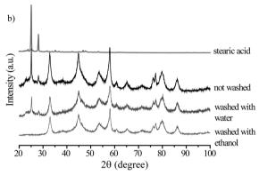
Fig. 8 ATR-IR spectra (a) and X-ray diffraction patterns (b) of a spent 1Pt/Al<sub>2</sub>O<sub>3</sub> catalyst after APR of a glycerol/methanol/Na oleate mixture (synthetic crude), before washing, washed with water and washed with ethanol and stearic acid for comparison
