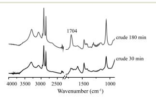
Fig. 9 ATR-IR spectra of a spent Pt/Al<sub>2</sub>O<sub>3</sub> catalyst after crude glycerol APR; after 30 min and after 180 min.
