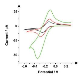
Fig. 1 Cyclic voltammograms recorded within 1 mM hexaammineruthenium(III) chloride/0.1 M KCl using unmodified (black line) and DMFmodified (10 minutes solvent immersion, 30 minutes of curing at 100 °C) ESPEs with (red line) and without (green line) an additional protecting DMF inert film over the insulating dielectric layer. Scan rate: 50 mV s<sup>-1</sup> (vs. SCE).
