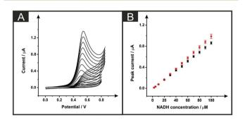
Fig. 5 Typical cyclic voltammograms (A) as a result of increasing concentrations of NADH (2.5–100  $\mu\text{M})/\text{pH}$  7.1 PBS using a DMF-modified ESPE (10 minutes within the solvent and a curing temperature of 100 °C for 30 minutes) and corresponding calibration plots (B) over the concentration range using an unmodified ESPE (squares) and DMF-modified ESPE (circles). Represented data indicate the average and standard deviations (N = 3). Scan rate: 50 mV s $^{-1}$  (vs. SCE).
