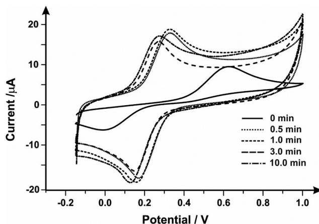
Fig. 1 Cyclic voltammetric responses obtained using a SPE in 1 mmol  $\text{L}^{-1}$  ammonium iron(II) sulfate/0.2 M  $\text{HClO}_4$  solution as a result of varying mechanical activation/polishing times using alumina slurry. Scan rate:  $50 \text{ mV s}^{-1}$  vs. SCE.
