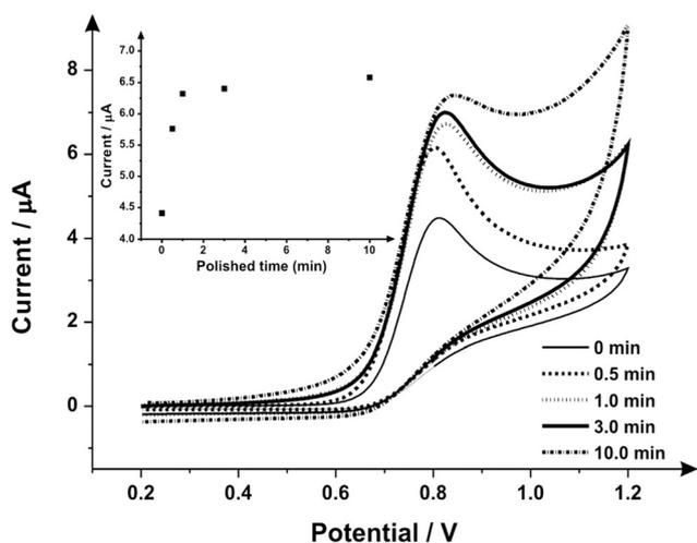
Fig. 3 Cyclic voltammetric study of the variation of mechanical activation/polishing times recorded in  $50 \mu\text{mol L}^{-1}$  sodium nitrite/PBS (pH 7) using SPEs (different SPE per experiment). Inset: a plot of current as a function of mechanical activation/polishing time (with alumina slurry) variation. Scan rate:  $50 \text{ mV s}^{-1}$  vs. SCE.
