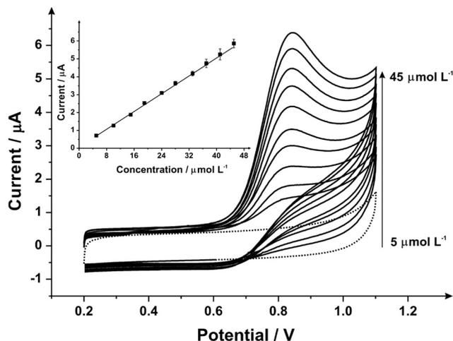
**Fig. 7** Cyclic voltammograms obtained from additions of sodium nitrite (5–45  $\mu\text{mol L}^{-1}$ ) into pH 7 PB using a 1 minute mechanically activated/polished SPE with diamond slurry using the same SPE throughout the experimentation (scan rate: 100  $\text{mV s}^{-1}$  vs. SCE); the dotted line represents the blank (no sodium nitrite) response. Inset: analysis of the voltammetric peak heights as a function of concentration.
