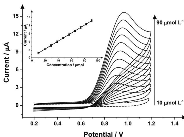
Fig. 4 Cyclic voltammograms obtained from additions of sodium nitrite ( $10\text{--}90 \mu\text{mol L}^{-1}$ ) into pH 7 PB using a 3 minute mechanical activation/polished SPE with alumina slurry using the same SPE throughout the experimentation (scan rate:  $100 \text{ mV s}^{-1}$  vs. SCE); the dotted line represents the blank (no sodium nitrite) response. Inset: analysis of the voltammetric peak heights as a function of concentration.
