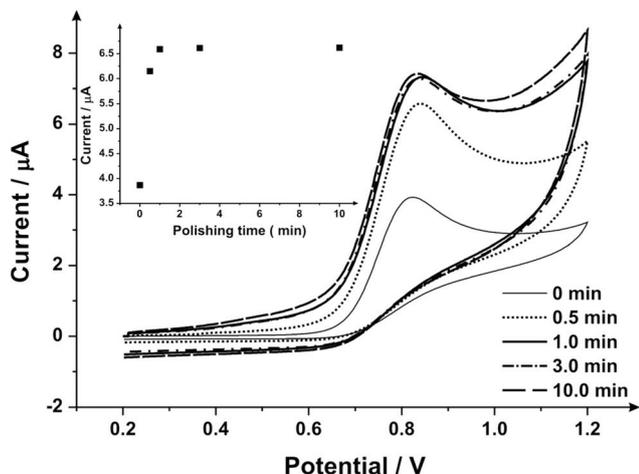
**Fig. 5** Cyclic voltammetric study of various mechanical activation/polishing times obtained in  $1 \text{ mmol L}^{-1}$  sodium nitrite/PBS (pH 7) using SPEs (different SPE per experiment). Inset: a plot of current as a function of the polishing time (with diamond spray) variation. Scan rate:  $50 \text{ mV s}^{-1}$  vs. SCE.
