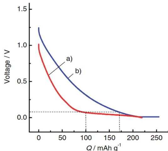
Fig. 19 Chronopotentiograms of the second reduction for hard-carbon electrodes in (a) 1 mol dm<sup>-3</sup> NaClO<sub>4</sub> and (b) 1 mol dm<sup>-3</sup> LiClO<sub>4</sub> PC solution in Na and Li cells, respectively, at a rate of 25 mA g<sup>-1</sup>. Reproduced with permission<sup>128</sup> © 2011, WILEY-VCH Verlag GmbH & Co.
