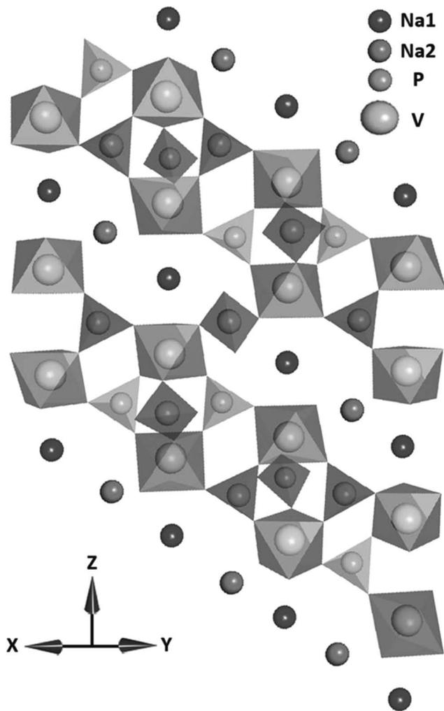
Fig. 9 The crystal structure of  $\text{Na}_3\text{V}_2(\text{PO}_4)_3$  in the  $a$  and  $b$  plane. Reproduced with permission<sup>81</sup> © 2013, WILEY-VCH Verlag GmbH & Co.
