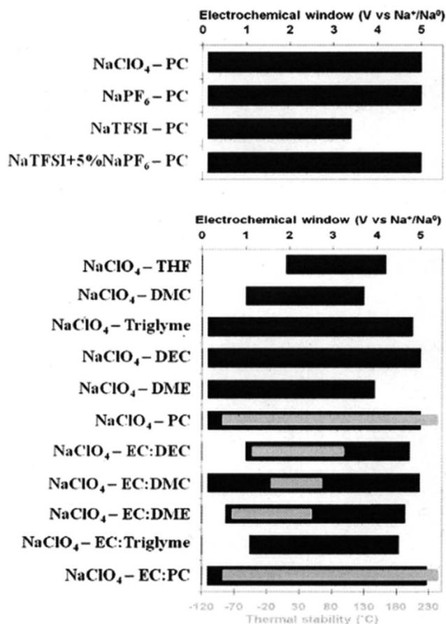
Fig. 15 Electrochemical potential window stability of various salts with PC and NaClO<sub>4</sub> in various solvents. Reproduced with permission<sup>150</sup> © 2012, RSC Publishing.
