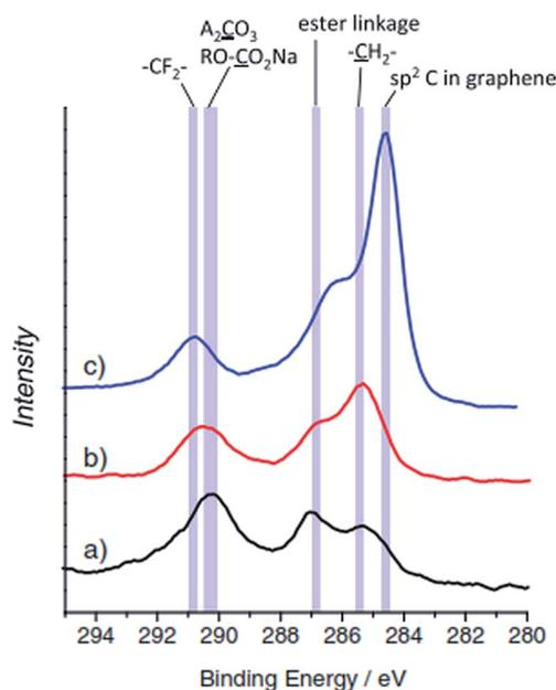
Fig. 20 XPS carbon 1s spectra for the hard-carbon electrodes tested in (a) sodium and (b) lithium cells after the first cycle, and (c) pristine electrode. Reproduced with permission<sup>128</sup> © 2011, WILEY-VCH Verlag GmbH & Co.
