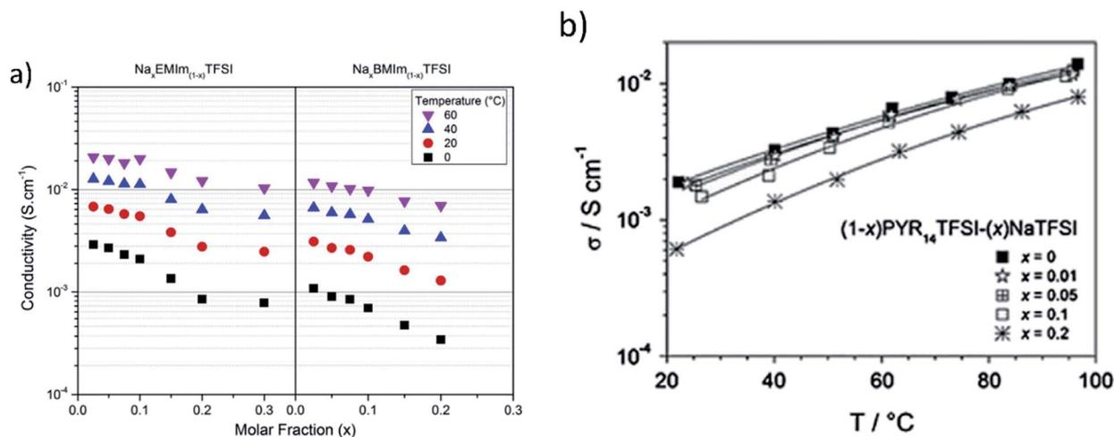
Fig. 18 (a) Isotherms of the conductivity as a function of the molar fraction of Na<sub>x</sub>-EMIm<sub>(1-x)</sub>TFSI and Na<sub>x</sub>BMIm<sub>(1-x)</sub>TFSI (reproduced with permission<sup>153</sup> © 2014, Elsevier) and (b) ionic conductivity vs. temperature for the (1 - x)PYR<sub>14</sub>TFSI-(x)NaTFSI electrolyte. Reproduced with permission<sup>154</sup> © 2014, Elsevier.
