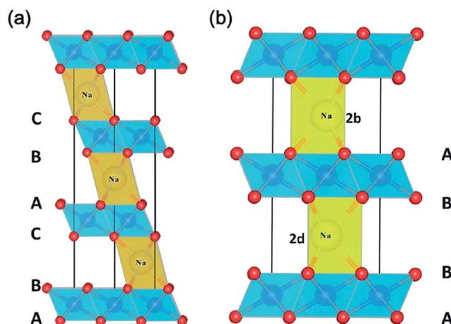
Fig. 3 The crystal structure of (a) O3 and (b) P2 phases in  $A_xMO_2$ . Reproduced with permission<sup>4</sup> © 2013, RSC Publishing.
