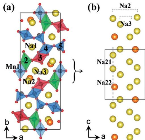
Fig. 5 (a) Crystal structure of  $\text{Na}_{0.44}\text{MnO}_2$  showing Mn and Na binding sites, and (b) the S shaped tunnel configuration along  $c$ -axis with different sodium positions Na21 and Na22 in  $\text{Na}_{0.44}\text{MnO}_2$ . Reproduced with permission<sup>35</sup> © 2012, ACS Publications.
