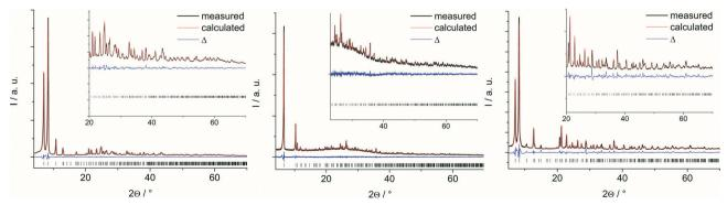
Fig. 2 Final plots of the Rietveld refinements of 1, 2 and 3 (from left to right). Measured data are shown as black lines and calculated fit as red lines; the blue curves indicate the difference plots. Vertical bars mark the allowed Bragg reflection positions
