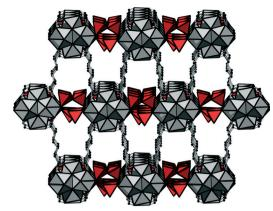
Fig. 7 Framework structure of 3 as seen along [110]. Guest molecules present inside the cavities are omitted for clarity. ZrO polyhedra are shown in grey, Cr<sub>2</sub>O<sub>7</sub><sup>2-</sup> ions in red and carbon atoms in black.
