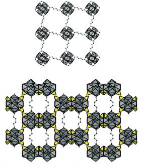
Fig. 5 Top: the square grid layer in 2 formed by the interconnection of inorganic nodes via adipate molecules, as seen along the c-axis. Bottom: the framework structure of 2 as seen along the a-axis. Guest molecules filling the channels are omitted for clarity. ZrO polyhedra are shown in grey, sulfate ions in yellow and carbon atoms in black.
