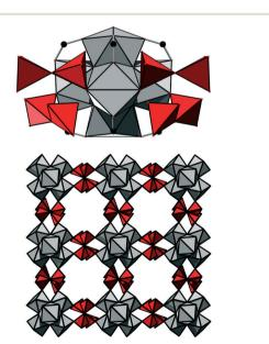
Fig. 6 Top: dichromate ions coordinated to the Zr cluster in a monodentate fashion. Bottom: the inorganic doubly connected square grid formed by the interconnection of Zr-oxo clusters and dichromate ions. Note that the positions of the dichromate ions are only partially occupied, adding up to 75%. ZrO polyhedra are shown in grey, Cr<sub>2</sub>O<sub>7</sub><sup>2-</sup> ions in red and carbon atoms in black.
