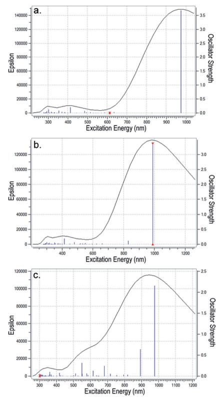
Fig. 7 The UV-vis spectra for (a) PEDOT $^{2+}$  (without PSS $^{2-}$  counterion); (b) PEDOT $^{2+}$  slightly bent to interact with the dianion; and (c) PEDOT $^{4+}$  with more bending when it interacts with the tetracation.
