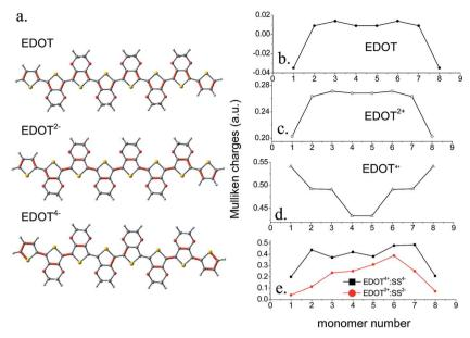
Fig. 5 (a) Nature of bond alternation in EDOT, EDOT $^{2+}$  and EDOT $^{4+}$ . The red bonds are aromatic double bonds (1.38–1.39 Å for C=C and 1.70 Å for C=S). (b) Mulliken charges for EDOT. (c) Mulliken charges for EDOT $^{2+}$ . (d) Mulliken charges for EDOT $^{4+}$ . (e) Mulliken charges for EDOT $^{2+}$  and EDOT $^{4+}$ -SS $^{4-}$ .
