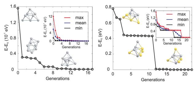
Fig. 2 Evolution of the lowest isomer for  $Ag_8$  (left) and  $Au_4Ag_4$  (right), relative to the energy of the GM isomer ( $E_0$ ). The lowest energy isomers for  $Ag_8$  ( $Au_4Ag_4$ ) from the initial, the 1st and the 5th (the initial, the 3rd and the 12th) generation are shown. In the inset the change of the lowest (min, black), averaged (mean, blue) and highest (max, red) lying isomers with generation is highlighted.
