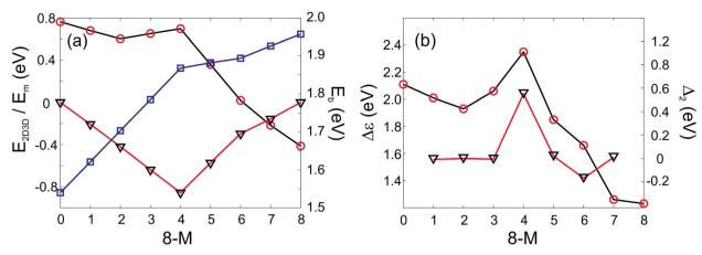
Fig. 5 PWscf calculated energies: (a) Energy differences between 2D and 3D isomers ( $E_{2D3D}$ , red circles), mixing energy ( $E_m$ , black triangles) and binding energies ( $E_b$ , blue squares); (b) HOMO–LUMO gap ( $\Delta \varepsilon$ , red circles) and second differences ( $\Delta_2$ , black triangles) as a function of the number of Au atoms. A positive value of  $E_{2D3D}$  means that the 3D structure is more stable.
