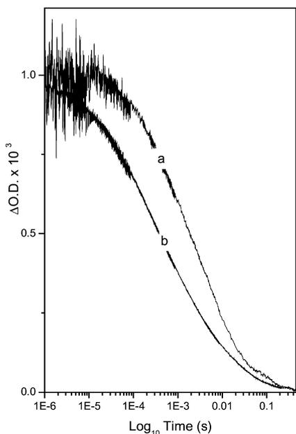
**Fig. 1** Transient absorption data probing the decay of photoinduced dye cation absorption (excitation 625 nm, probe 800 nm) at room temperature for (a) an Al<sub>2</sub>O<sub>3</sub>/TiO<sub>2</sub>/RuL<sub>2</sub>(NCS)<sub>2</sub> film and (b) a TiO<sub>2</sub>/RuL<sub>2</sub>(NCS)<sub>2</sub> film. The decay dynamics are assigned to the recombination reaction (3) in Scheme 1.
