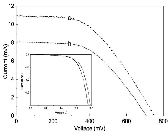
**Fig. 2** Photocurrent–voltage curves of DSSC with (a) and without (b) the incorporation of an Al<sub>2</sub>O<sub>3</sub> overlayer under AM 1.5 irradiation. The inset illustrates the dark current in both samples.
