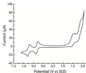
Fig. 4. Cyclic voltammogram of free base porphyrin **20** in dichloromethane obtained under the conditions described in the text.
