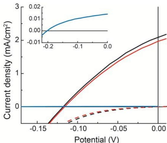
**Fig. 7.** Current density-voltage plots for DSSC with SnO<sub>2</sub> photoanodes sensitized by **7** (red) and **4** (black). The solid lines show performance under illumination (simulated AM 1.5 G solar irradiation) and the dotted lines show behavior in the dark. The blue curve shows the behavior of a DSSC using **7** deposited on a TiO<sub>2</sub> electrode. The inset is an expansion of the vertical axis for **7** on TiO<sub>2</sub>.
