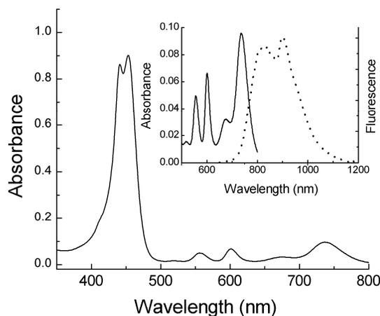
Fig. 5. Spectrum of **13** in dichloromethane. The inset shows absorbance (solid line), and fluorescence with excitation at 451 nm (dotted line).
