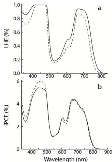
**Fig. 6.** (a) Light-harvesting efficiency (LHE) of  $SnO_2$  electrodes bearing **7** (dashed) and **4** (solid). The absorption spectra were corrected by subtraction of the spectra of the corresponding unsensitized electrodes. (b) Incident photon to current efficiency (IPCE) as a function of wavelength for DSSC constructed using the electrodes whose LHE are shown in (a). The curves are from electrodes bearing **7** (dashed) and **4** (solid).
