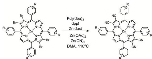
Fig. 1. General synthetic scheme for cyanation of  $\beta$ -bromoporphyrins.
