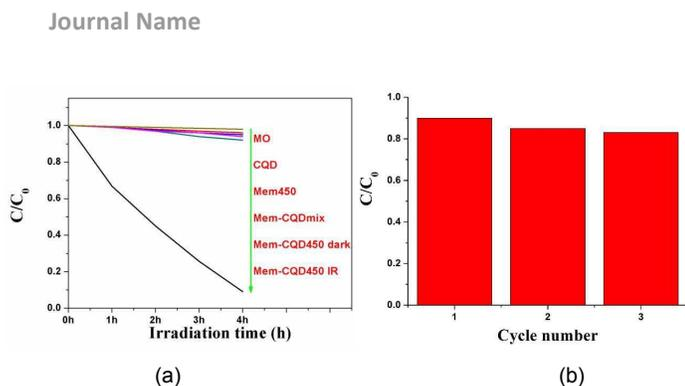
**Fig 5.** (a) The photodegradation of methyl orange (4 mg/L) by CQD, Mem450, Mem-CQDmix and Mem-CQD450 under infrared light irradiation ( $\lambda > 800$  nm), respectively; (b) The reusability test of Mem-CQD450 photocatalyst under infrared light irradiation ( $\lambda > 800$  nm).
