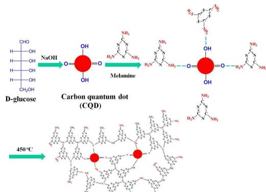
**Fig 3.** The proposed mechanism for synthesizing Mem-CQD450 composite.
