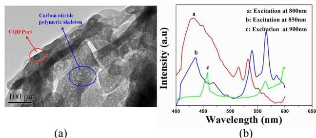
**Fig 4.** (a) TEM image of Mem-CQD450 at 100 nm scale; (b) Photoluminescence spectra of Mem-CQD450 at the excitation wavelength 800, 850 and 900 nm, respectively.
