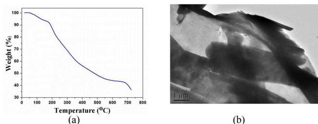
**Fig 2.** (a) Thermogravimetric analysis of CQD; (b) TEM image of CQD treated at 450 °C for 2 h.
