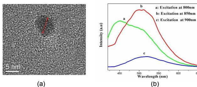
**Fig 1.** (a) TEM image of CQD at 5 nm scale; (b) Photoluminescence spectra of CQD at the excitation wavelength of 800, 850 and 900 nm, respectively.
