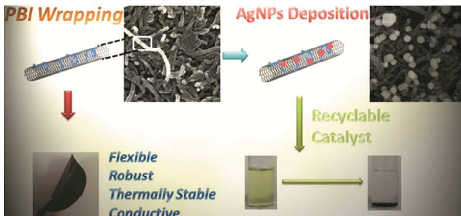
Multi walled carbon nanotube buckypapers and their hybrids with Ag nanoparticles have been fabricated with the assistance of polybenzimidazole.
