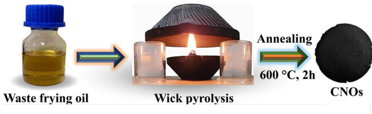
Fig. 6 A schematic illustration for the synthesis of CNOs by flame pyrolysis method 76
