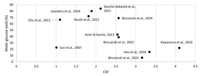
Combined severity factor (CSF) vs. glucose yield of the acid hydrolysis studies.
