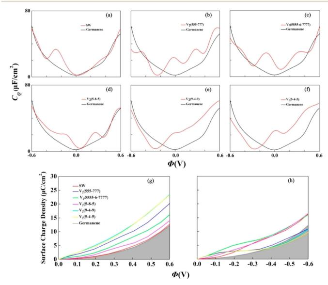
Fig. 2 (a-f)  $C_Q$  for pristine Ge-ene and defective Ge-ene; (g and h) surface charge density variation with respect to potential drop having  $\Phi$  in the range of 0.0 to 0.6 V and -0.6 to 0.0 V. The results were evaluated in the supercell 6  $\times$  6 and it possesses a defect concentration of 1.39%. Reproduced with permission from ref. 33. Copyright (2020), the American Chemical Society.
