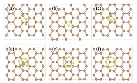
Fig. 14 Structure optimized for pristine  $\beta$ -Sb with the PBE functional for (a) Li<sub>2</sub>S@Sb, (b) Li<sub>2</sub>S<sub>2</sub>@Sb, (c) Li<sub>2</sub>S<sub>4</sub>@Sb, (d) Li<sub>2</sub>S<sub>6</sub>@Sb, (e) Li<sub>2</sub>S<sub>8</sub>@Sb, and (f) S<sub>8</sub>@Sb. Reproduced with permission from ref. 51. Copyright (2021), the American Chemical Society.
