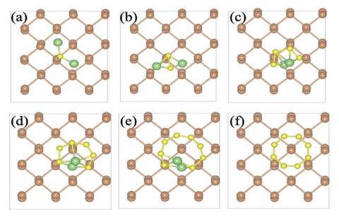
Fig. 13 Structure optimized for pristine  $\alpha$ -Sb with the PBE functional for (a) Li<sub>2</sub>S@Sb, (b) Li<sub>2</sub>S<sub>2</sub>@Sb, (c) Li<sub>2</sub>S<sub>4</sub>@Sb, (d) Li<sub>2</sub>S<sub>6</sub>@Sb, (e) Li<sub>2</sub>S<sub>8</sub>@Sb, and (f) S<sub>8</sub>@Sb. Reproduced with permission from ref. 51. Copyright (2021), the American Chemical Society.
