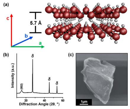
Fig. 5 (a) Pictorial representation of the stacked structure of Ge; (b) XRD spectrum of Ge, showing a stacking peak present at  $\sim$ 15.4° and other peaks represent characteristic Ge elemental impurities; (c) SEM image of Ge. Reproduced with permission from ref. 41. Copyright (2017), the American Chemical Society.
