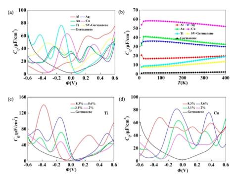
Fig. 3 (a) Calculated  $C_{\mathbb{Q}}$  of the SV Ge-ene with the given elements adsorbed and the SV Ge-ene with respect to the local electrode potential  $(\Phi)$ ; (b) change in  $C_Q$  over the temperature range of 0-400 K; calculated  $C_Q$  of the SV Ge-ene with respect to (c) Ti and (d) Cu doping with concentrations of 2%, 3.1%, 5.6%, and 8.3% with respect to local electrode potential. Reproduced with permission from ref. 33. Copyright (2020), the American Chemical Society.
