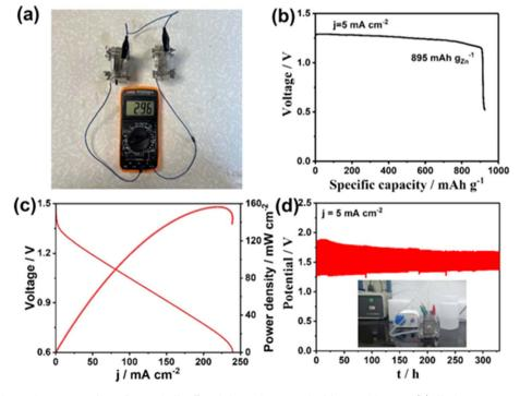
Fig. 12 (a) OCV for the series connection of two similar Zn-air batteries tested with a multimeter; (b) discharge curve at a constant current density of 5 mA cm<sup>-2</sup>; (c) polarization curve and power density of Zn-air battery with respect to different current densities; (d) stability test performed for the Zn-air battery for 329 h (inset: digital photograph of the battery cycling). Reproduced with permission from ref. 48. Copyright (2024), the American Chemical Society.
