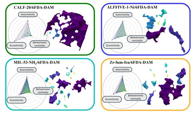
Fig. 5 3D visualizations of the interfacial pore networks for CALF-20 (green), ALFFIVE-1-Ni (blue), MIL-53-NH<sub>2</sub> (cyan) and Zr-fum-fcu (yellow) composites, highlighting differences in pore connectivity and distribution. Radar plots summarize three key graph theory network parameters: assortativity, eccentricity, and betweenness centrality
