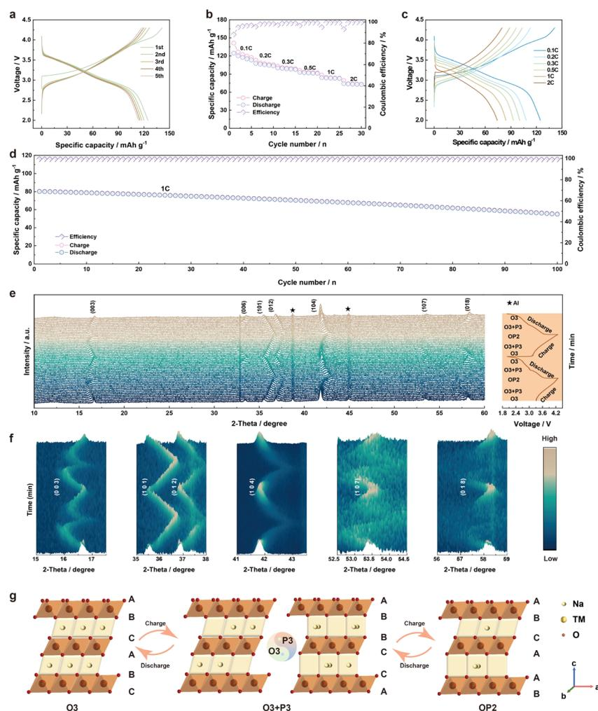
Fig. 6 Electrochemical performance of NaFM-F within the potential window of 2–4.3 V (a) GCD curves at 0.1 C. (b) Rate performance. (c) GCD curves at different rates. (d) Cycling performance at 1 C. (e) *In situ* XRD patterns of NaFM-F in the first two cycles at 0.1 C in the potential window of 2.0–4.3 V. (f) The corresponding contour plots. (g) Schematic diagram of the structural evolution process during the Na<sup>+</sup> extraction/insertion.
