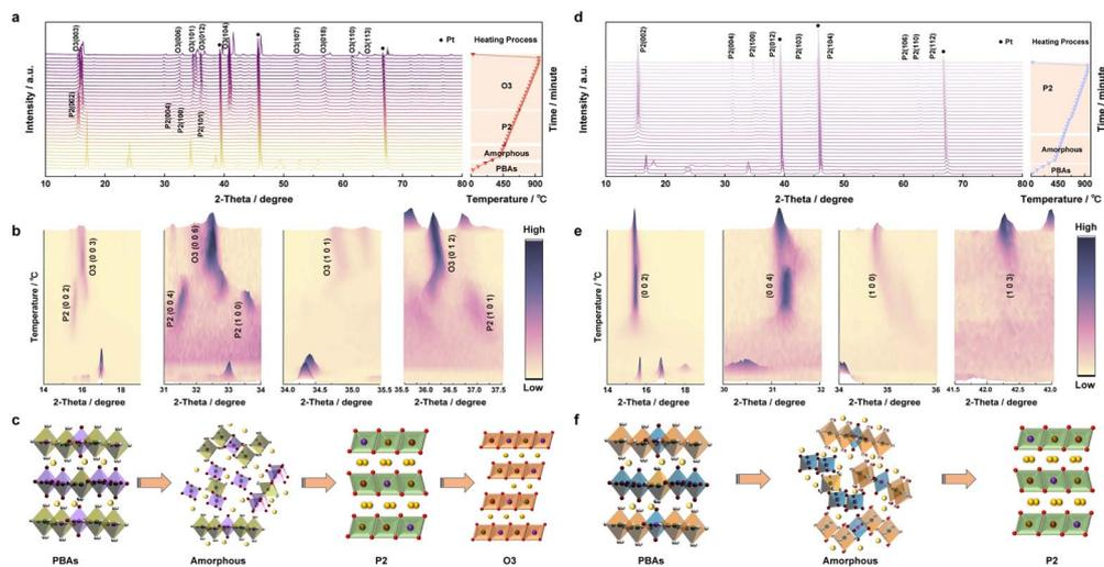
Fig. 2 *In situ* HTXRD patterns of the process (a) from PBAs-NFM to NaFM and (d) from PBAs-FM to NaFM. The corresponding main characteristic diffraction peak intensity contour maps (bird's eye view) of the process (b) from PBAs-NFM to NaFM and (e) from PBAs-FM to NaFM. Schematic diagram of the transformation process (c) from PBAs-NFM to NaFM and (f) from PBAs-FM to NaFM.
