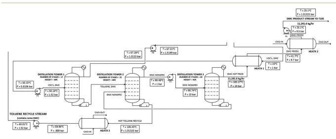
Fig. 5 PFD of the solvent recovery and DMC purification step of the process.
