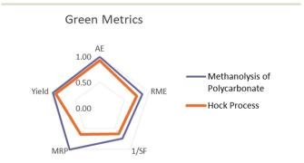
Fig. 6 The comparison of the green metrics for the methanolysis of polycarbonate and the Hock process.
